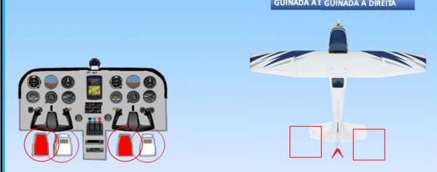
The slide shows a cockpit instrument panel on the left with red circles around the rudder pedals. On the right, a top-down view of a white airplane shows the rudder deflected to the right, with red boxes around the rudder and the tail section.
