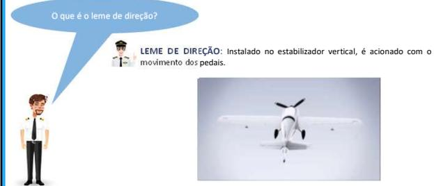
The slide features a cartoon pilot on the left with a speech bubble asking 'O que é o leme de direção?'. To the right, a small icon of a pilot is next to the text definition. Below the text is a top-down view of a white airplane with the rudder highlighted.
