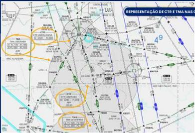
The diagram shows a portion of an ENRC (Brazilian Aeronautical Information Publication) map. It highlights the boundaries of Terminal Manoeuvring Areas (TMA) and Control Zones (CTR) around several airports. The map includes various flight paths, altitudes, and other aeronautical data. The TMA and CTR areas are circled in yellow.
