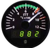
A circular gauge with a black face and white markings. The scale ranges from 0 to 12, with major ticks every 2 units and minor ticks every 0.2 units. The needle is currently pointing to approximately 8.8. The text 'ITT' and '°C x 100' are printed on the gauge. Below the gauge, there is a digital display showing '882'.
