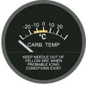
A circular gauge with a black face and white markings. The scale ranges from -20 to 20 degrees Celsius, with major ticks every 10 units and minor ticks every 2 units. The needle is currently pointing to approximately 10°C. The text 'CARB. TEMP' is printed below the scale. Below the gauge, there is a warning: 'KEEP NEEDLE OUT OF YELLOW ARC WHEN PROBABLE ICING CONDITIONS EXIST'.
